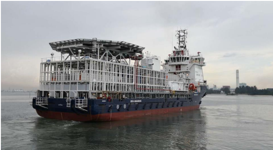
Plate 3.2: Typical Node deployment vessel with On-Board Equipment
