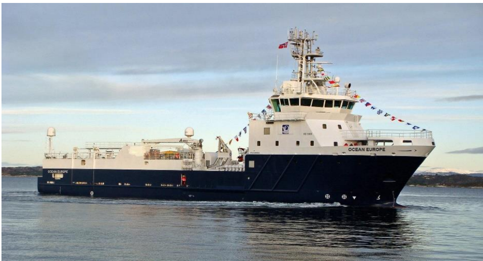
Plate 3.3: Typical Source (Air Gun Shooting) Vessel
