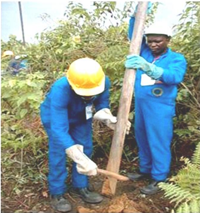
Plate 5.2: Thumping shallow pattern holes (Removing debris)
