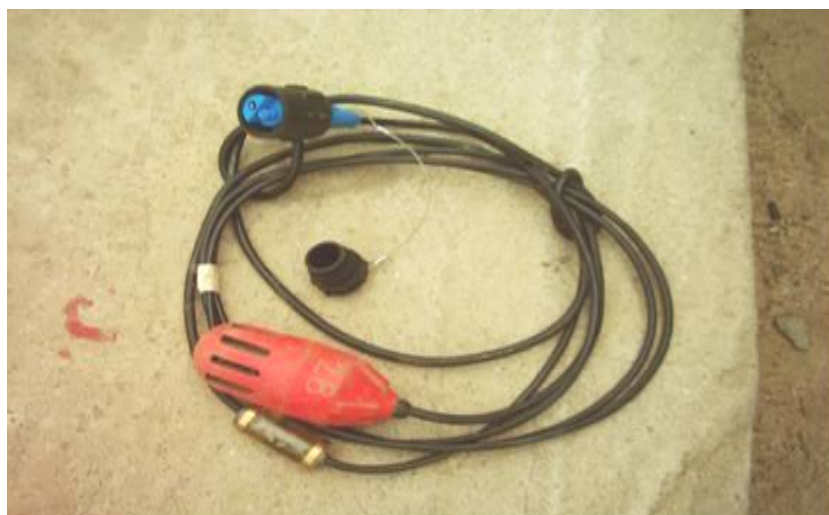
Plate 3.11: A typical Hydrophone proposed to be used during the Seismic survey
