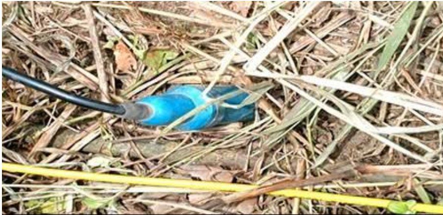
Plate 3.9: A typical Geophone used for detecting signals on land
